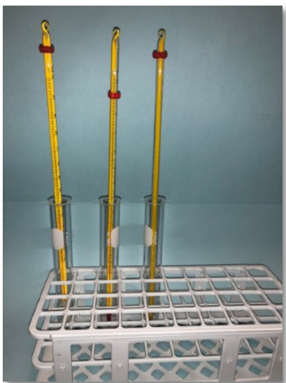
Fig. 3 Thermometers with towels attached placed in test tubes.
